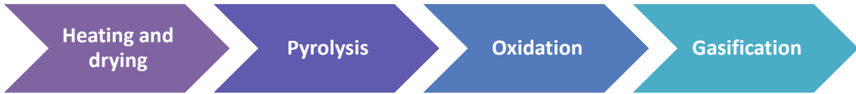
Figure 4 Gasification process steps (Source: Ruiz, 2013)
